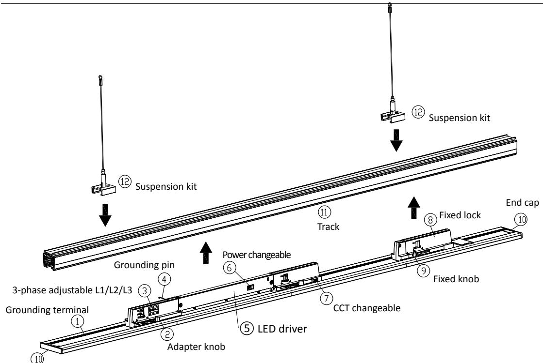
**Step 1:** In ⑥ power selection, set the power through DIP switch; On the ⑦ dial color adjustment switch, provide a switch to set color temperature (only for adjustable color models)
