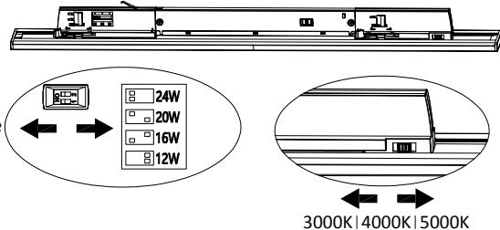
**Step 2:** Select the corresponding phase/circuit mode through DIP switch in ③ phase selection;
