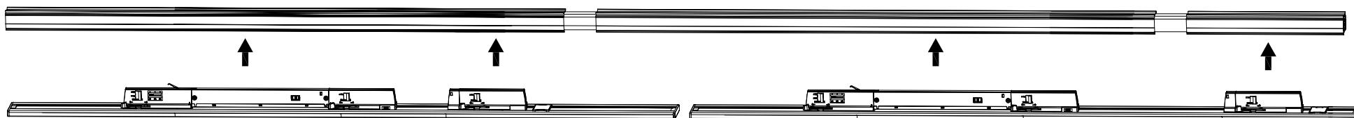
**Step 2:** Install the lighting fixtures onto the track
