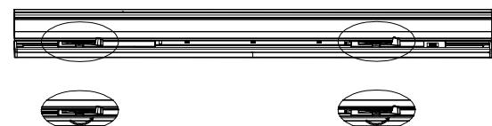
**Attention:** Pay attention to the positioning knob and do not install it in reverse! Incorrect installation may result in irreparable damage.
